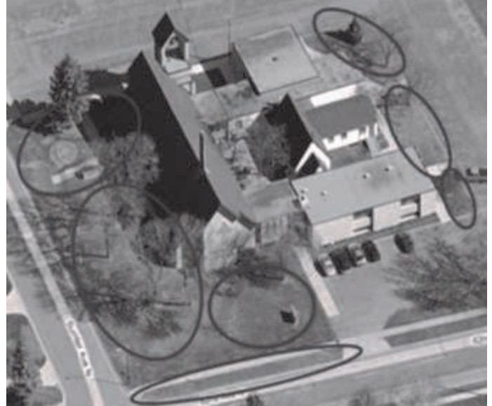
Aerial view of First Lutheran Church of Crystal. Circled areas indicate proposed sprinkler zones.
